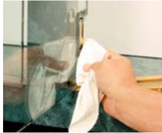
Block the door to maintain alignment and remove the cover plate. Clean glass in gasket area.
