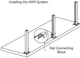
**2C.** ✓ Cut Elevated Bottom Rail to length. Mount the Bottom Rail onto the Blocks and secure with Cat. No. TEK1 Tek Screws.
