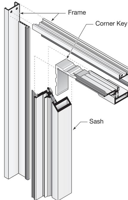
When closed, the vent is sealed to the frame with E.P.D.M. bulb gaskets ensuring an air tight seal. The 1" (25) laminated glazing is held in place with structural silicone.
