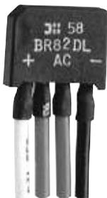
2 amp rated rectifier converts low voltage AC current DC of same voltage.
