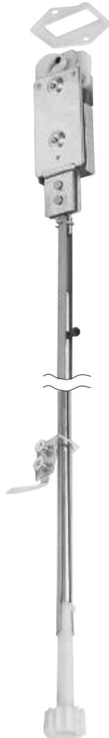
Our DL2240 Series Header Bolt is designed to add a top-door locking point in the inactive door. This bolt is activated when the DL2110B or MS18533 Latch is locked. As the throw bolt locks into the inactive door, it lifts the adjustable nylon rod end causing the Header Bolt to lift and expand its pawls in the head, which centers the bolt into the header. One per package.
