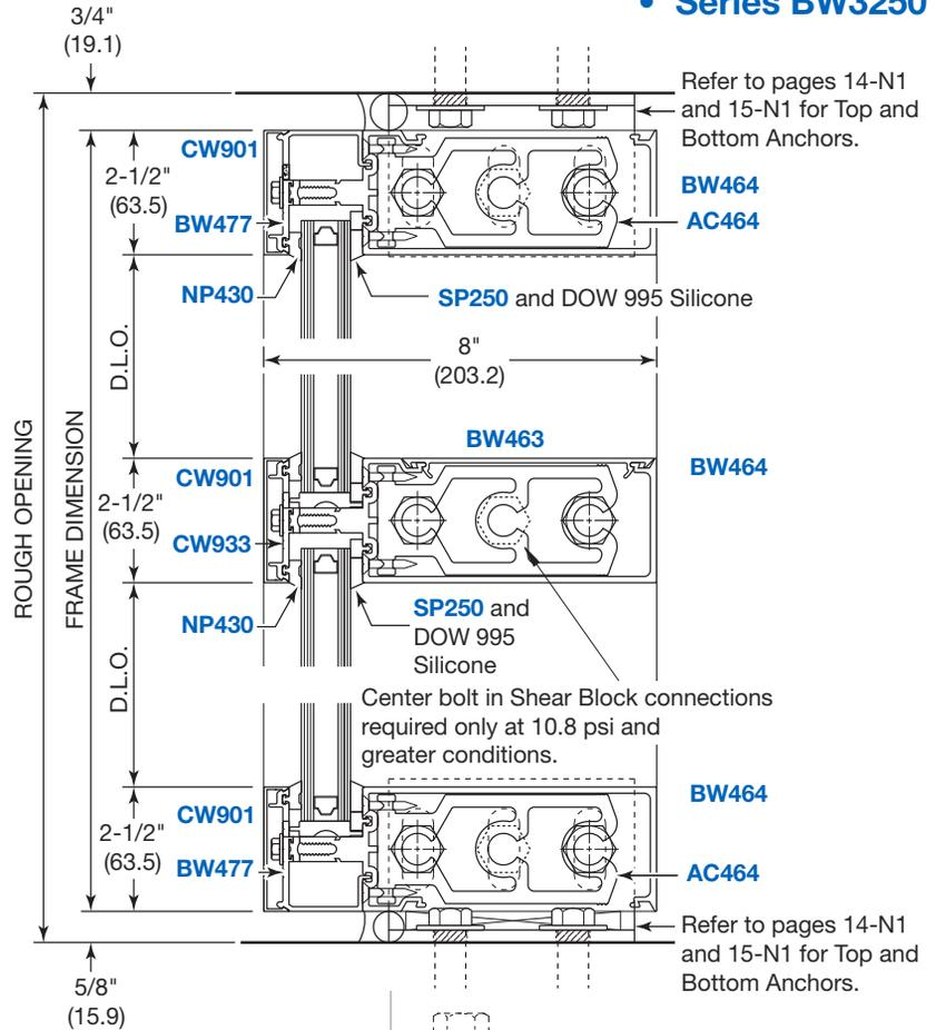
Center bolt in Shear Block connections required only at 10.8 psi and greater conditions.
