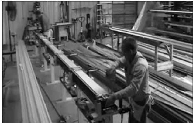
1. With the pneumatic clamping system on, set the jigs to their proper locations and begin fastening Shear Blocks to one side of the Curtain Wall's Vertical Mullion. Proceed down the Vertical Mullion until all Shear Blocks are installed.
