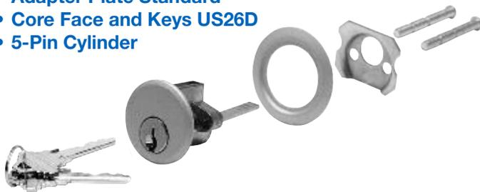
This Rim Cylinder comes with two keys in the Schlage "C" keyway configuration. 1-7/8" (47.6) break-away screws and 1-1/4" (31.8) break-away spindle standard. They are available keyed different or keyed alike in satin aluminum or dark bronze finishes. One per package.
