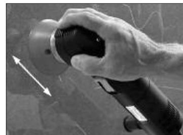
Work the polishing head, very slowly, with consistent pressure for 30 seconds, and then stop. Inspect the progress of your work. Repeat until scratch is removed.
