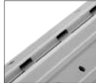
Standard Duty Hinges have 16 load bearing blocks for doors up to 200 pounds (90 kg). Heavy-Duty Hinges have 32 load bearing blocks for doors up to 600 pounds (272 kg) if attached with Riv-Nuts®.
