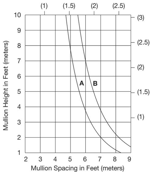
Deadload charts are based on 1/8" (3.2) maximum deflection at the center point of the horizontal member and on a glass weight of 6.5 psf (31.74 Kg/m<sup>2</sup>). Glass shall rest on two setting blocks located at:
