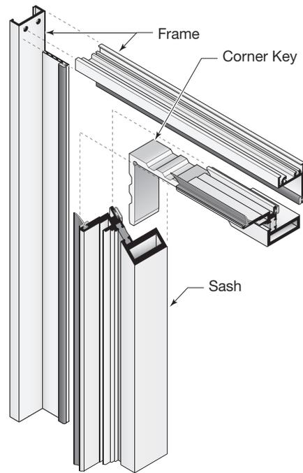
When closed, the vent is sealed to the frame with E.P.D.M. bulb gaskets ensuring an airtight seal. The glass is held in place with structural silicone. The Series 7500 Concealed Vent is available in 1" (25) or 1/4" (6) glass versions.
