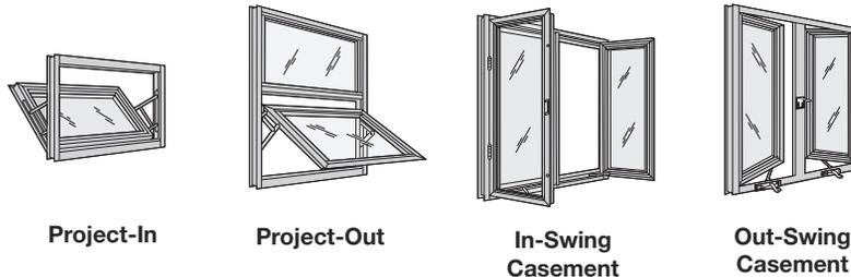
Projected and casement windows operate by moving away, or "projecting," from the window frame, as awning or hopper vents, and as in-swinging or out-swinging casement vents. Projected windows open and close horizontally while casement windows operate on a vertical axis.
