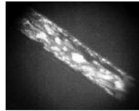
**LIGHT SURFACE or SCUFF MARK SCRATCH** – Over 95% of all scratches are light scratches or scuff marks. This magnified image above shows a light scratch. This scratch can be removed.
