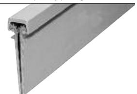
These U.S. Aluminum Concealed Leaf Continuous Hinges have load bearing blocks every 5-1/8" (130.2) on the Standard Duty Hinge, and every 2-9/16" (65.1) on the Heavy-Duty Hinge. They are available in satin anodized and dark bronze anodized finishes, and stocked in 83" (2.11 m) lengths. A pack of installation screws is included with each Hinge. Replacement Screw Packs are also available separately.
