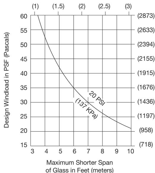
Stress on structural silicone should not exceed 20 psi (137 KPa) for a 6:1 safety factor.
