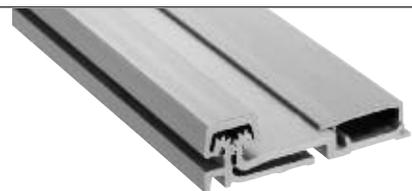
These U.S. Aluminum Full Surface Continuous Hinges have load bearing blocks every 5-1/8" (130) on the Standard Duty Hinge, and every 2-9/16" (65) on the Heavy-Duty Hinge. They are available in satin anodized and dark bronze anodized finishes, and stocked in 83" (2.11 m) lengths. A pack of installation screws is included with each Hinge. Replacement Screw Packs are also available separately.
