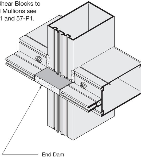
Injected Molded End Dams are for controlling any infiltrated water. Apply sealant to three contact sides of End Dams and slide between vertical and horizontal joints as shown.
