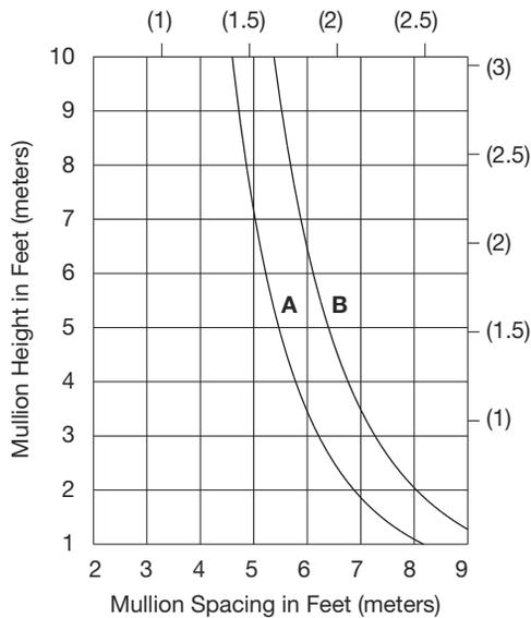
Deadload charts are based on 1/8" (3.2) maximum deflection at the center point of the horizontal member and on a glass weight of 6.5 psf (31.74 Kg/m<sup>2</sup>).
