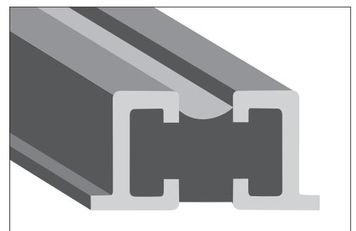
Channel with polyurethane thermal break
