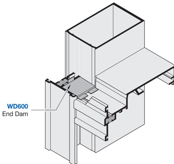
Injected Molded End Dams are for controlling any infiltrated water. Apply sealant to the four contact sides of end dams and slide between vertical and horizontal joint as shown. See page 17-J6 for additional information.
