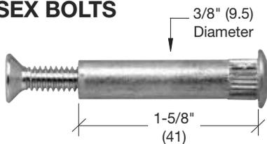
Used for securing push bars, surface mounted door closers, and other fixtures to 1-3/4" (44.5) doors. Knurled barrel fits a 3/8" (9.5) diameter hole. Available in aluminum and bronze finishes. Four bolts per package.
