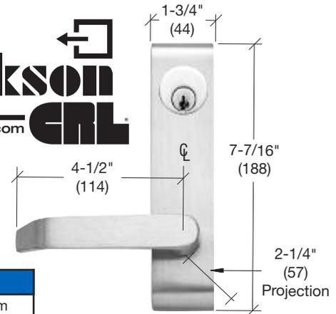
The Jackson Locking Flat Lever Outside Trim has a narrow 1-3/4" (44) escutcheon that allows it to be used on narrow stile doors. The flat style lever is key-controlled, and requires the use of our Part No. DRA10 Series Keyed Mortise Cylinder, which locks or unlocks the lever (ANSI Function – 08)
