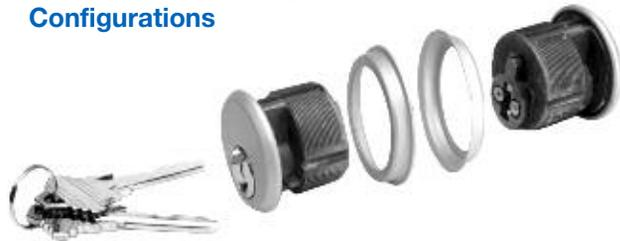
Our Double Mortise Key Cylinder comes with two keys in either Schlage "C" or Yale "8" keyway configurations. 1-5/32" (29.4) diameter, 1" (25) long 5-Pin Cylinder; AR MS – Type Cam; Core Face and Keys US26D. Die cast zinc construction. Includes 3/16" (4.8) cylinder rings. One pair per package.
