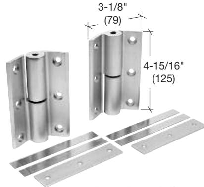
This Universal Hinge Replacement Kit is machined to the close tolerances required for heavy, continuously used commercial doors. The universal fit allows replacement of all storefront hinges without modification on both flush and 1/8" (3) recessed doors. The secure, non-exposed hinge pins cannot be reached, removed or tampered with. The door weight is supported by a case hardened, self-lubricating pin and machine quality anti-friction roller with thrust bearings sealed in oil.
