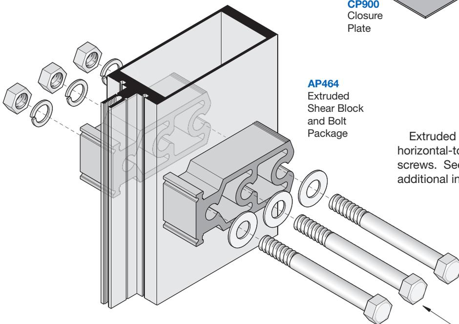
Center bolt in Shear Block connections only required at 10.8 psi conditions.
