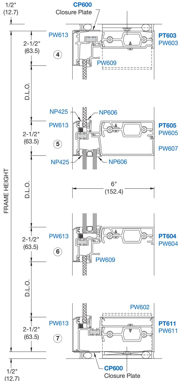
**NOTE:** The **PW613** Beveled Face Cap (shown) is Standard for Horizontal Members. The **CW901** Square Face Cap is Optional.
