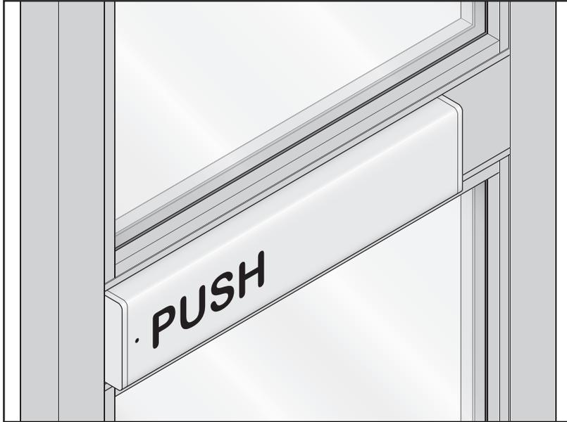
Combining contemporary styling with maximum security features, the Mid-Panel Panic option provides a Concealed Vertical Rod Panic Device with a Touch Bar Actuator. Matching mid-panels without hardware are available for sidelites.
