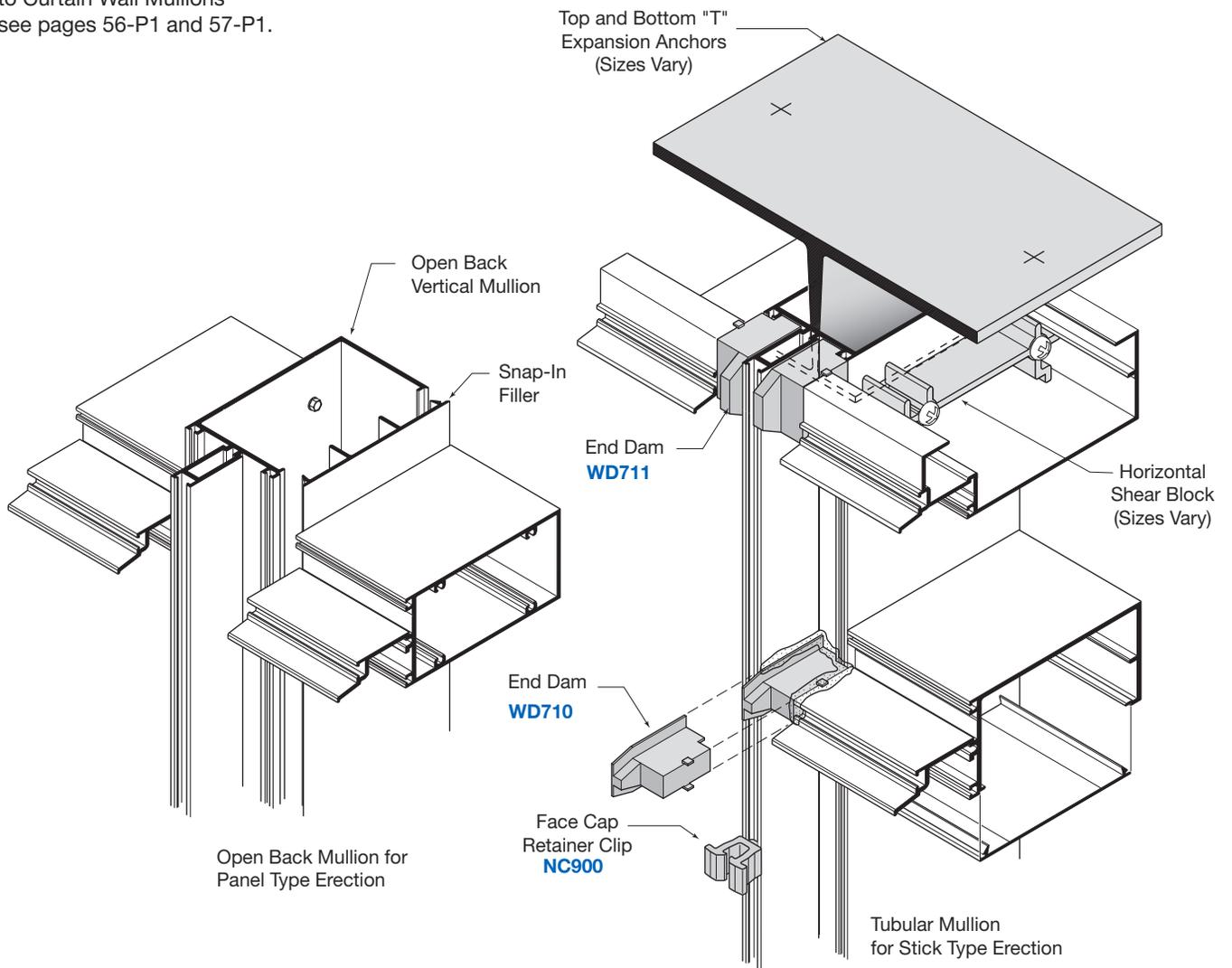
The two-piece vertical adds the versatility of screw race joinery and panel installation for window wall applications. A tubular horizontal attaches to the vertical and filler plate through screw splines. Open back head and sill horizontals allow for easy access for anchorage.
