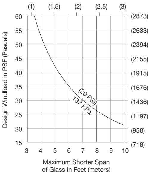
Stress on structural silicone should not exceed 20 PSI (137 KPa) for a 6:1 safety factor.
