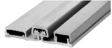
These U.S. Aluminum Full Surface Continuous Hinges have load bearing blocks every 5-1/8" (130.2) on the Standard Duty Hinge, and every 2-9/16" (65.1) on the Heavy-Duty Hinge. They are available in satin anodized and dark bronze anodized finishes, and stocked in 83" (2.11 m) lengths. A pack of installation screws is included with each Hinge. Replacement Screw Packs are also available separately.
