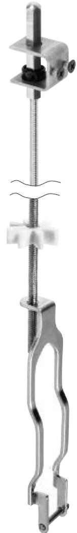
The AR4016 Series Header Bolt Kit is designed to add a top-of-door locking point for pairs of doors in the active leaf. Use with MS18533 Deadlocks. Designed for use on 84" (2134) tall doors which have the cylinder location no lower than 35" (889) from the floor. One per package. **NOTE:** Adams Rite Header Bolt Kit will not work with our DL Series Locks.
