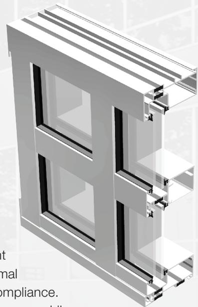
The Series OST451 Thermal Storefront System is engineered for optimal thermal performance and California Title 24 compliance. Offset glazing produces a flush appearance, while a slim 2" face trim and 4-1/2" depth offers a material cost advantage. The OST451 Storefront is a straight cut and stack system. No notching is required, which expedites installation and reduces labor.
