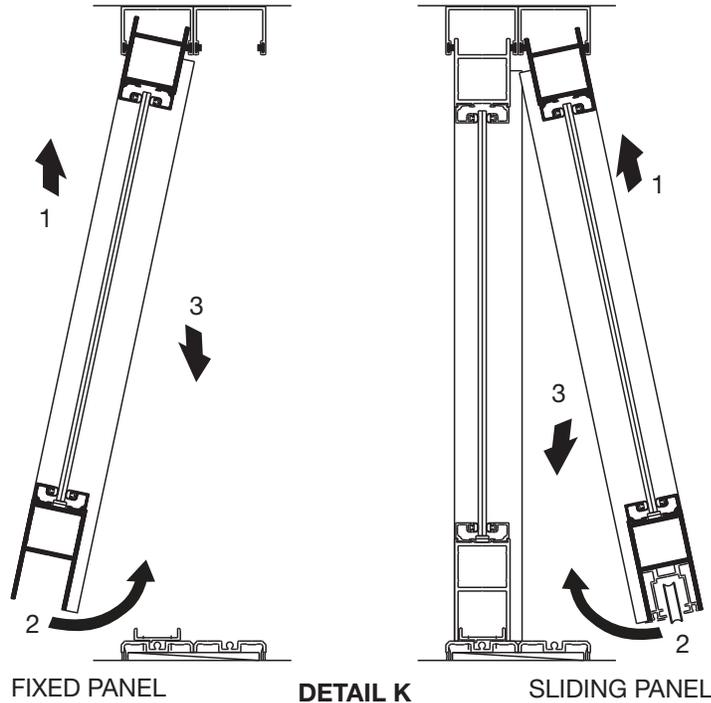
3. Remove SP237 Nylon Plugs from bottom of stiles. Adjust rollers through holes on both stiles to align panels and ensure proper engagement of hookbolt lock. Turn adjusting screws clockwise to raise panel and counterclockwise to lower it. **See DETAIL L.** Reinstall SP237 plugs.
