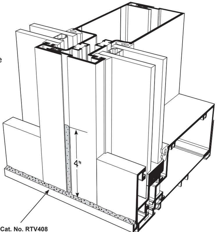
**CRITICAL SEAL:** Use **Cat. No. RTV408 Silicone Sealant** to seal along the exterior Subsill and into gaps between vertical mullions.
