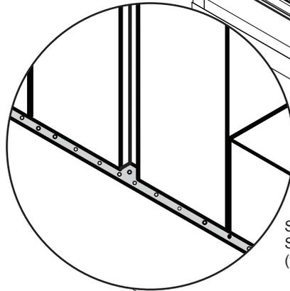
Seal between frames and Subsill for 8 pounds (test pressure) of water.
