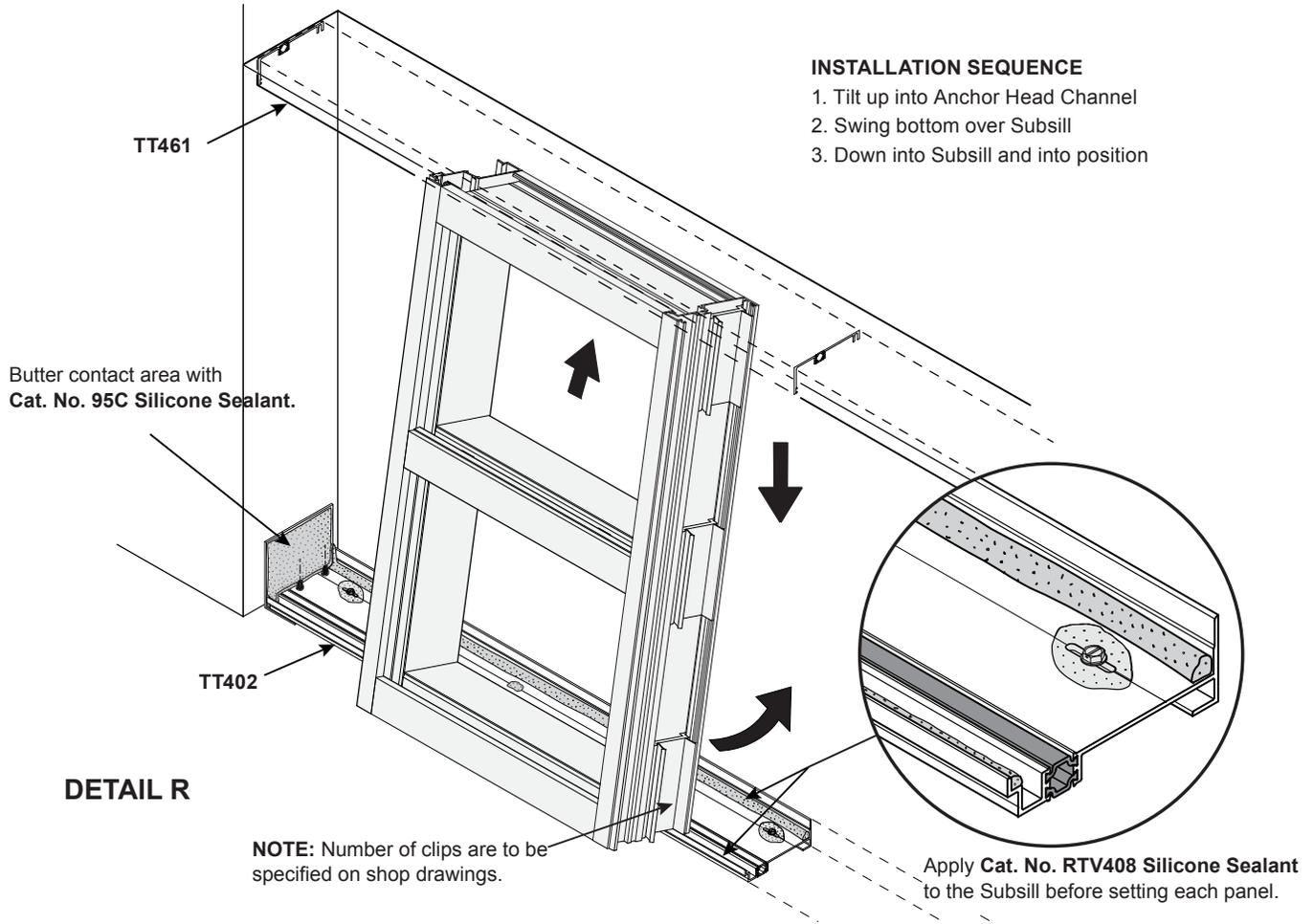
2. Slide Jamb against wall. Install next window and slide to snap into place.
