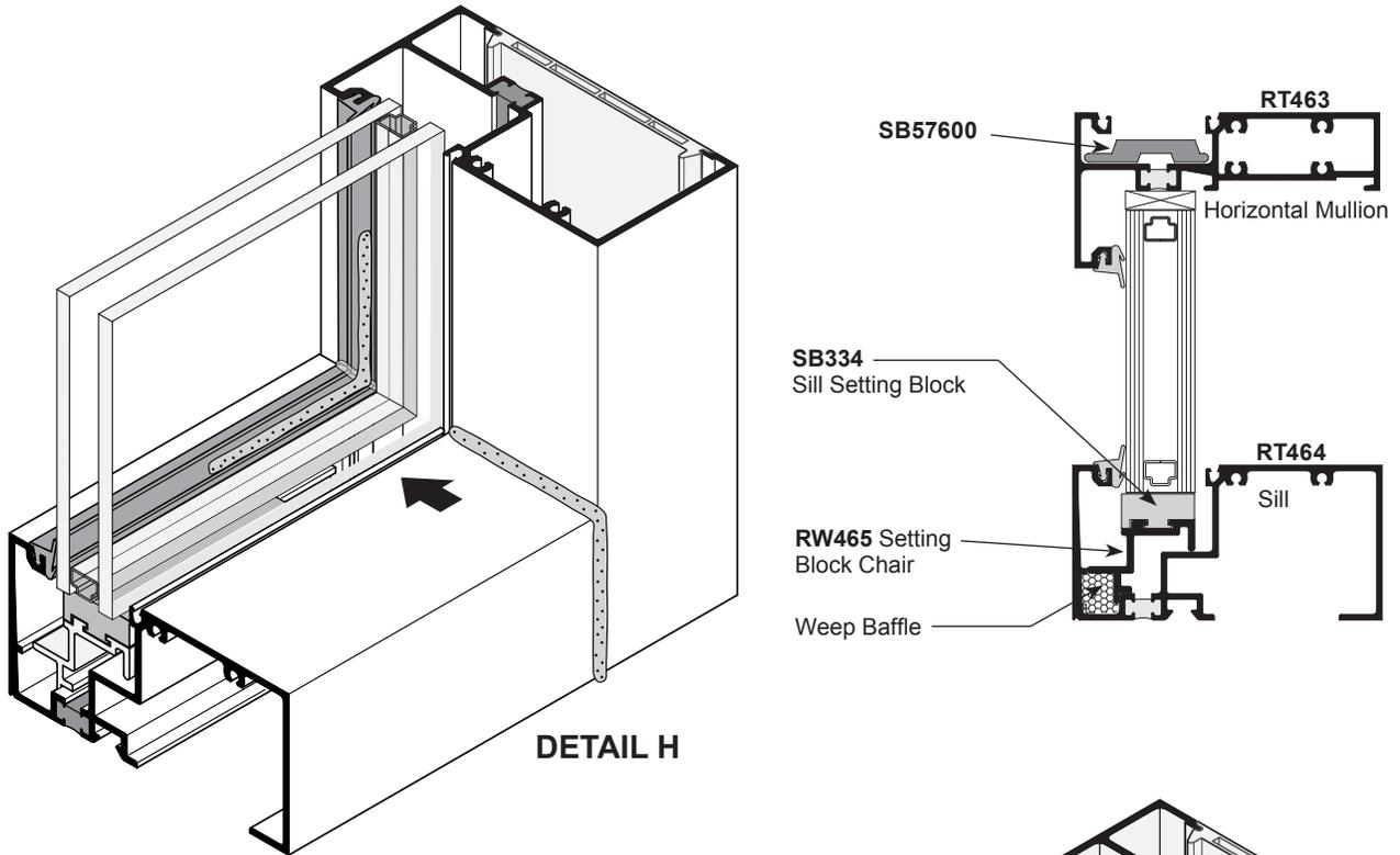
13. Push in temporary short wedges of the **NP225 Gasket** to hold glass in place.
