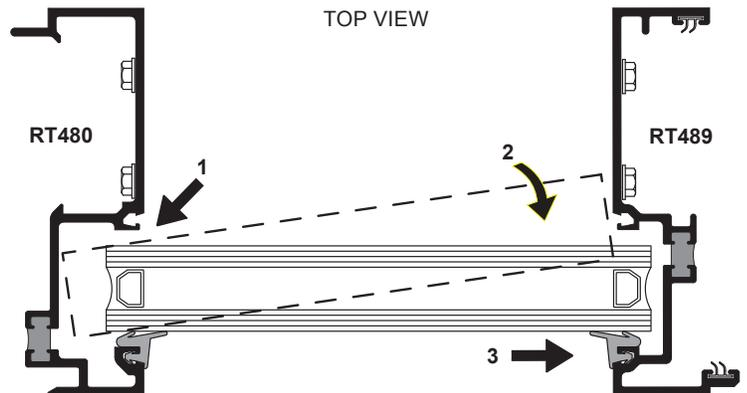
Install glass panel into frame by first angling the panel into the deep pocket. Swing the other end around and into the shallow pocket. Lower the panel down onto the setting blocks.
