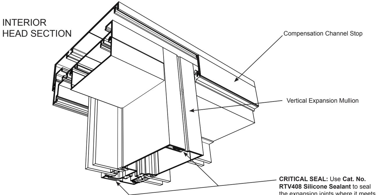
Apply **Cat. No. RTV408 Silicone Sealant** between all vertical expansion joints **BEFORE** attaching the Compensation Channel Stop. Additionally, all connection joints of vertical members that will be covered by the Compensation Channel Stop should be filled with sealant. This includes jambs, mullions, splayed verticals and SG joints.
