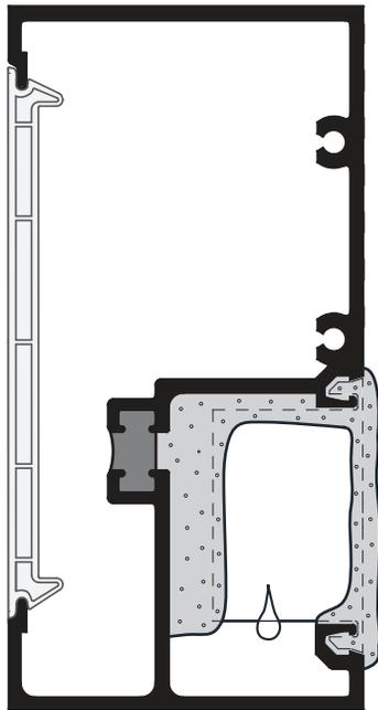
Apply **Cat. No. RTV408** Silicone Sealant to two sides of Glazing Pocket at Vertical and Horizontal Joint before inserting Water Deflector.
