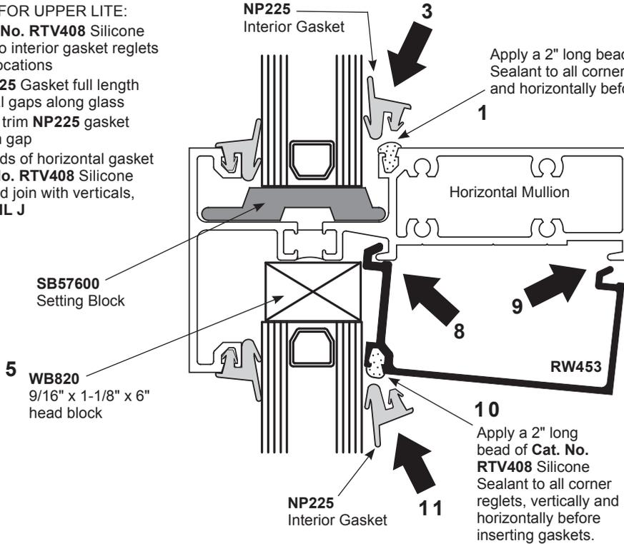
Apply a 2" long bead of **Cat. No. RTV408** Silicone Sealant to all corner gasket reglets, both vertically and horizontally before inserting gaskets.
