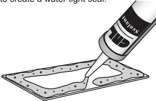
Run a 3" tall bead of silicone above the Subsill for 12 pounds (test pressure) of water.
